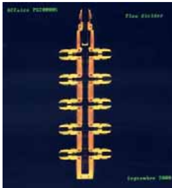
Part internals check by tomography
