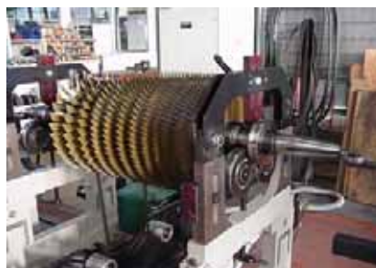
Centaur compressor being balanced
